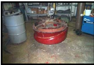
All molds are designed, constructed, and maintained by Hammond Roto-Finish. All molds are stored indoors to eliminate moisture contamination and UV attack.
