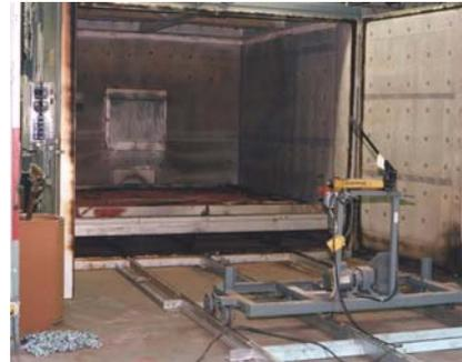
This will ensure that the bowl weldment integrity will remain intact during this process. Unlike others who may use a torch to remove the lining, we do not experience hot spots. Hot spots can cause warpage and metal fatigue.
